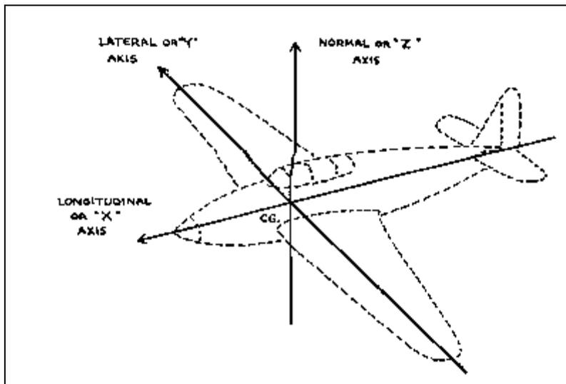
**Figure 10 The Axes of the Airplane**
